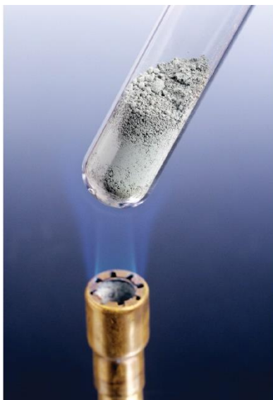
FIGURE 1 When heating a test tube, be sure to point it away from you or anyone else close by.
