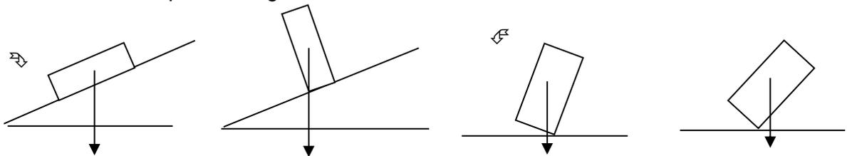
A structure is stable if the centre of mass is over the base. The width of the base and the height of the centre of mass affect the stability of a structure. To increase the stability, the centre of mass can be lowered and the width of the base increased.
