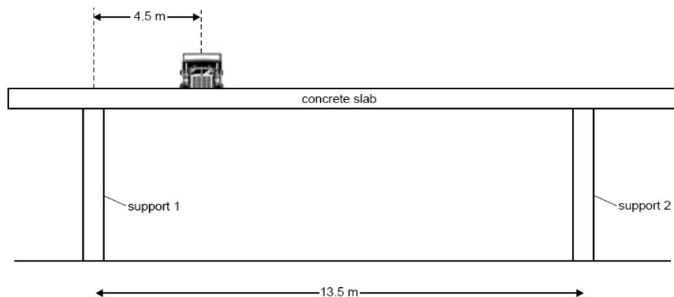
The figure above shows the front-on view of a loaded truck crossing a uniform concrete slab inside a building. The mass of the slab is 300 tonne, and the mass of the loaded truck is 50.0 tonne.
