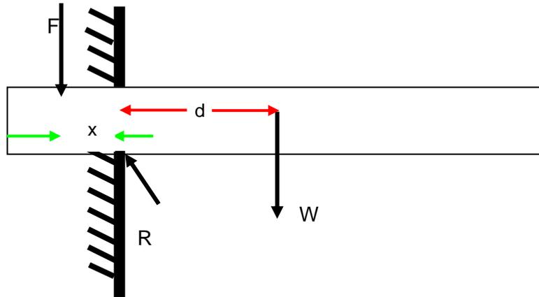
For this cantilever to be in equilibrium, the sum of the torques must be equal to zero, and the sum of the forces must equal zero. If we resolve the moments around the point that it will pivot from, ie. where  $R$  is acting. The clockwise moments =  $W \times d$ , and the anticlockwise moments are  $F \times x$ .
