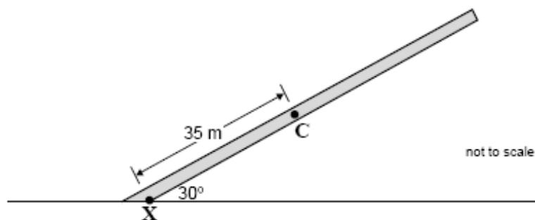
The centre of mass of the beam, C, can be considered to be 35 m from point X as shown.
