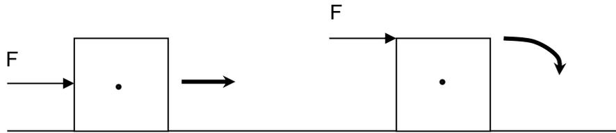
The turning force is most effective when it is acting at right angles to the rotating object. For example the turning force in the second diagram below produces more torque.
